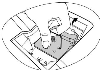
7. Tighten the screw that secures the lamp.
